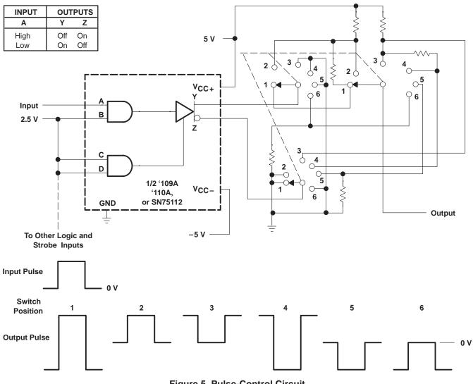
Figure 5. Pulse-Control Circuit
